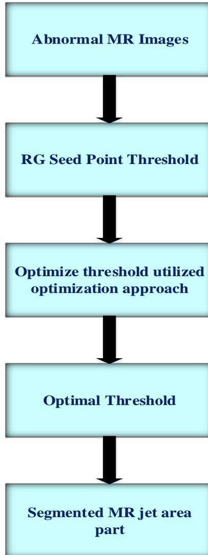
**Fig.3.3 Block diagram for the steps involved in segmentation process**
