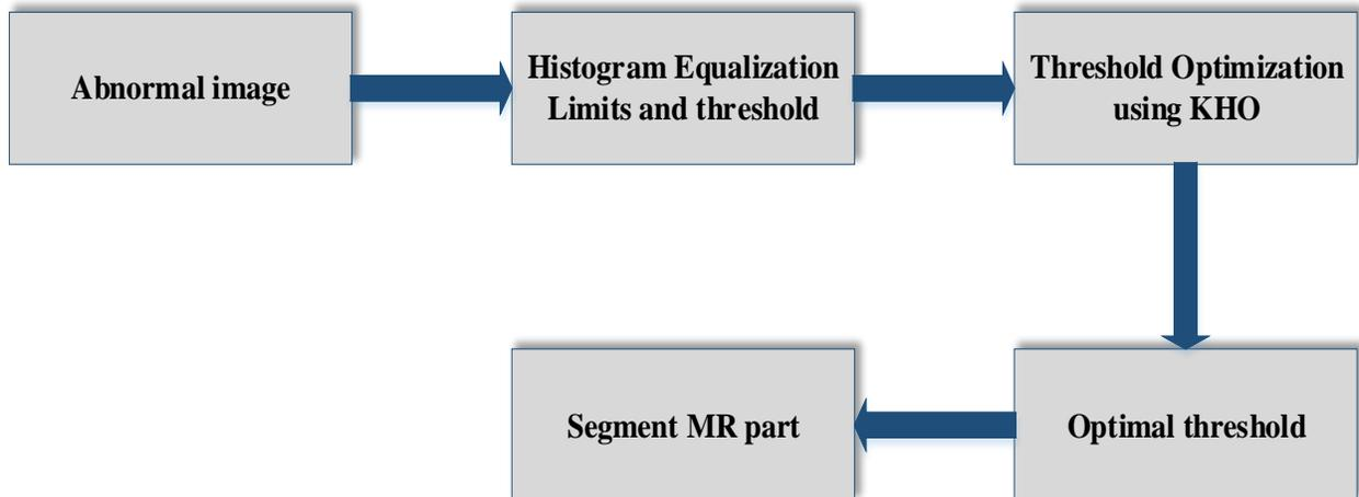
**Fig.4.2 Block Diagram for the Segmentation Process**
